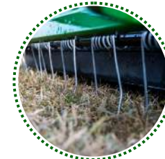
Rake Tine Bar Designed for effective dethatching to promote healthier turf.
